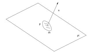
Claim 6.6. The stress at P across the surface perpendicular to  $\bf n$  is
