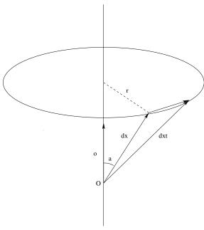
In fact, since  $\omega \times \Delta x$  is orthogonal to the plane determined by  $\omega$  and by  $\Delta x$ , it is tangent to the circle with center along the axis  $O\omega$  and radius determined by  $\Delta x$ . Moreover,
