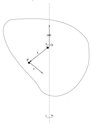
Then the **angular momentum** of an infinitesimal region of M around P is
