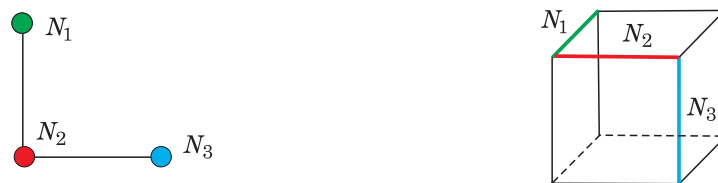
Figure 6. Interval graph and corresponding maximal intervals of a Boolean function f(x_1, x_2, x_3) .
