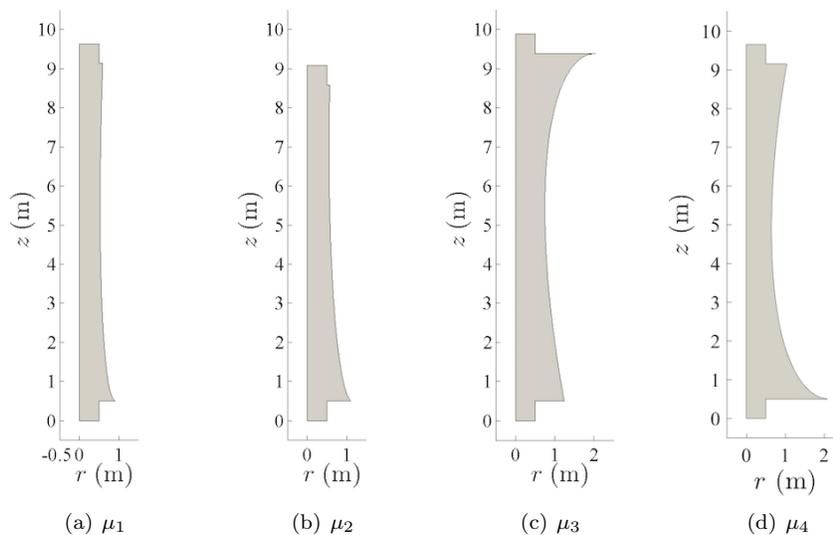
FIGURE 6. Shape of the optimized reactors,  $\Omega(\tilde{\phi}^{3,\text{opt}})$ , where  $\tilde{\phi}^{3,\text{opt}}$  is the solution of problem (3.9).
