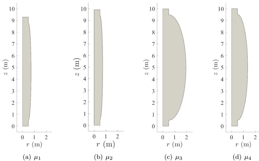
FIGURE 5. Shape of the optimized reactors,  $\Omega(\tilde{\phi}^{2,\text{opt}})$ , where  $\tilde{\phi}^{2,\text{opt}}$  is the solution of problem (3.6).
