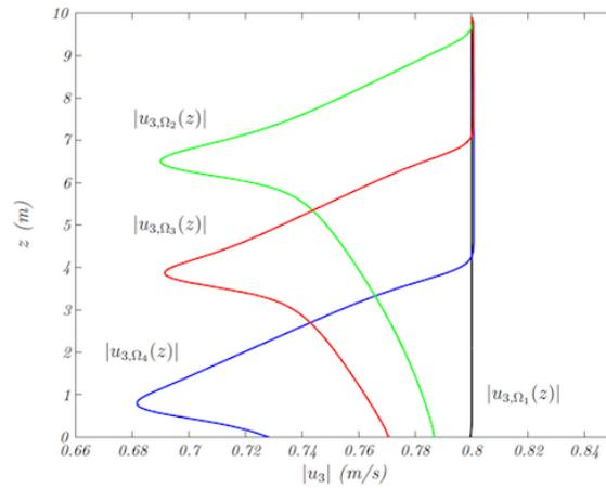
(e) Vertical velocity profile along the symmetry streamline obtained for reactor domains  $\Omega_i$ ,  $i = 1, \dots, 4$ .
