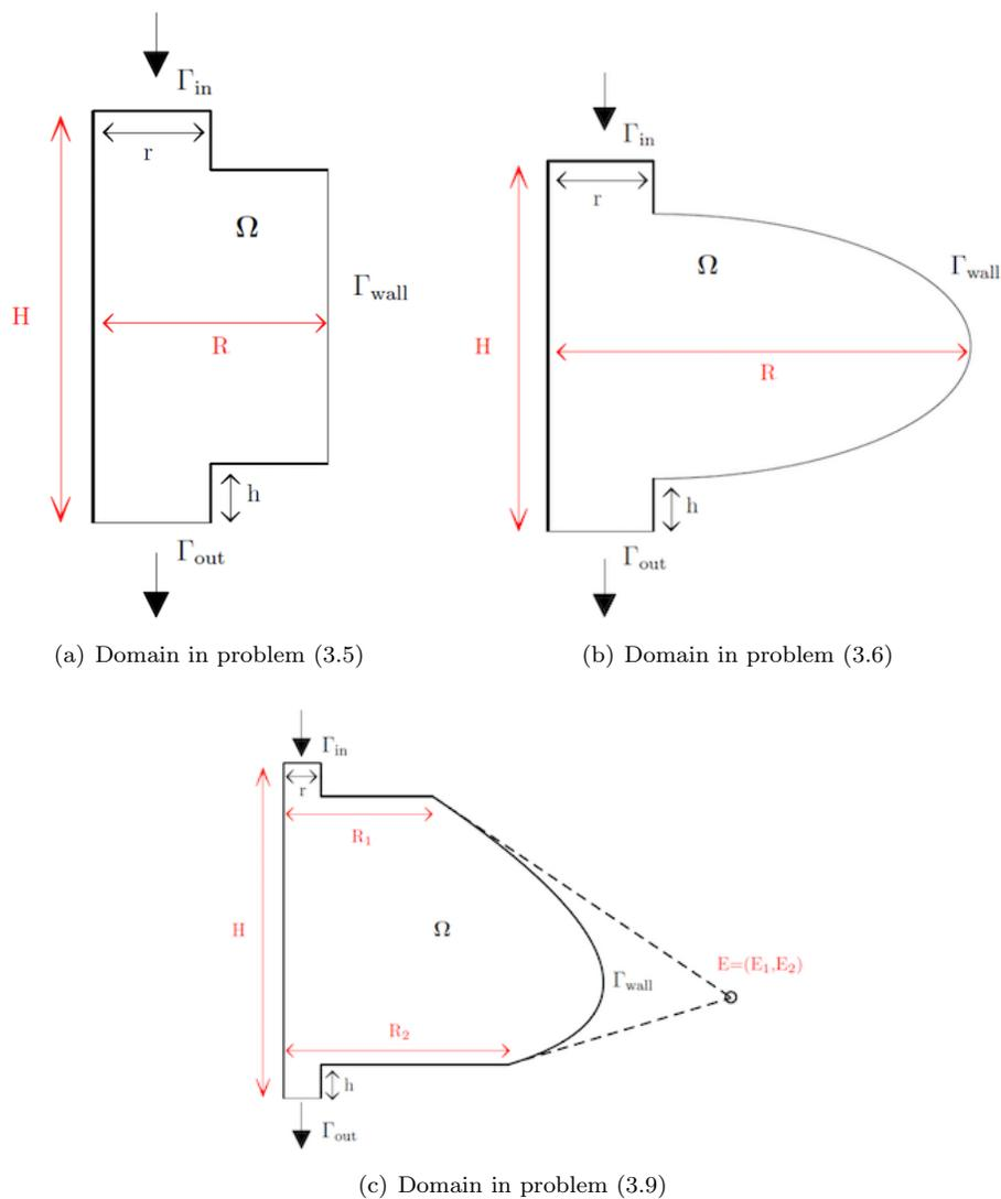
FIGURE 2. Schematic representation of the bioreactor geometries used to solve the discrete problems (3.5), (3.6) and (3.9).
