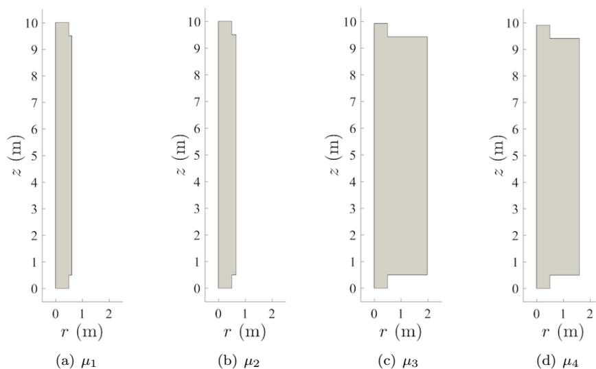
FIGURE 4. Shape of the optimized reactors,  $\Omega(\tilde{\phi}^{1,\text{opt}})$ , where  $\tilde{\phi}^{1,\text{opt}}$  is the solution of problem (3.5).
