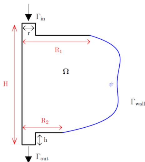
FIGURE 1. Schematic representation of the bioreactor geometries used to solve problem (3.1). The exterior curve (depicted in blue), which corresponds to part of the bioreactor exterior wall, is defined as  $(z, \psi(z))$ , where  $z \in [h, H - h]$ .
