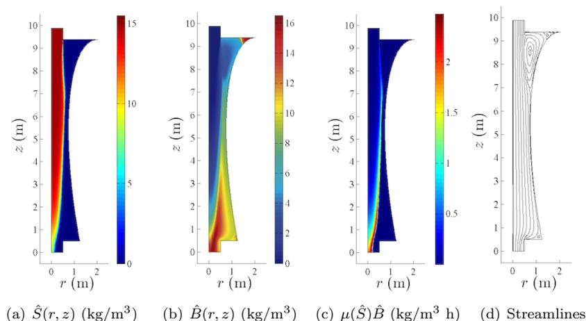
FIGURE 8. (a) substrate concentration (at steady state). (b) biomass concentration (at steady state). (c) reaction (at steady state) (d) streamlines. (a)-(d) associated with the optimal reactor  $\Omega(\phi^{3,\text{opt}})$  obtained for the growth rate function  $\mu_3$ .
