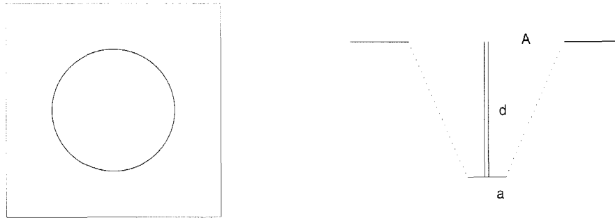
FIGURE 2.1 Schematic illustration of the force-displacement experiments performed on the outer capsule membrane. The capsule originally occupies a circle of radius A in its unstressed state, clamped between two steel plates (the left hand figure is a plan view). It is deformed into a shape that looks roughly like a truncated cone (right hand figure) by displacing a circular probe of radius a vertically through a distance d as shown.
