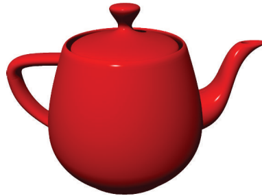
Figure 5: Teapot defined by 32 approximately implicitized patches from Section 8.3, with degrees given in Table 4 and ray traced using POV-Ray [25].
