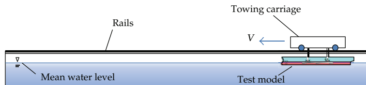
Figure 4: Layout of ocean engineering basin at the University of Tokyo.
