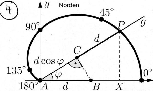
(b)  $\cos \varphi = \frac{|AC|}{|AB|}$   $|AC| = \underbrace{|AB| \cos \varphi}_d$   $|AP| = d \cos \varphi + d = d(1 + \cos \varphi)$
